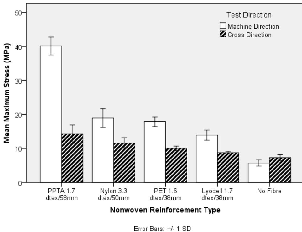
**Figure 3.** Tensile Strength of nonwoven-reinforced TPU composites
