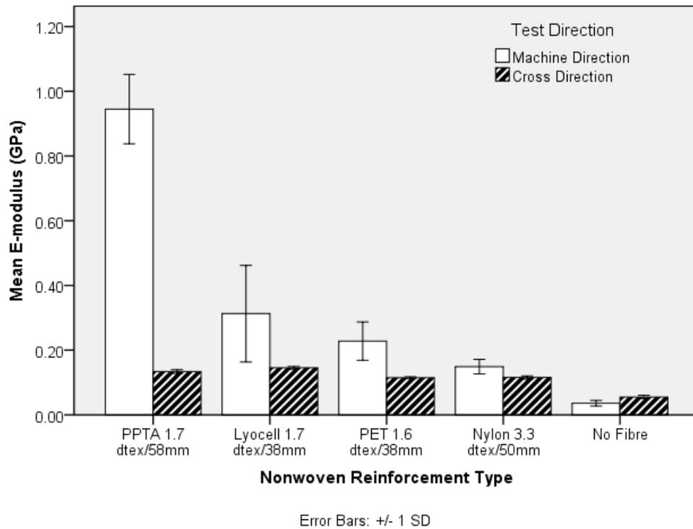
**Figure 4.** Tensile modulus of studied flexible composites
