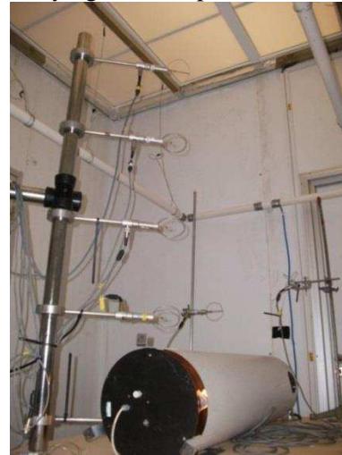
Figure 4 Anemometry results with patient and nurse heatloads, central extract 33 Hz supply fan. Cantilever anemometry pole measuring above DIN-man
