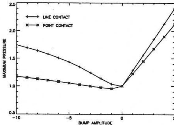
Figure 4 Comparison of maximum pressure between dented line and point contact, as a function of the amplitude.  $\mathcal{A} < 0$ : dent,  $\mathcal{A} > 0$ : bump,  $p_h = 3.0 \text{ GPa}$ ,  $b = 0.3 \text{ mm}$ ,  $\lambda = 0.5 \text{ mm}$ .
