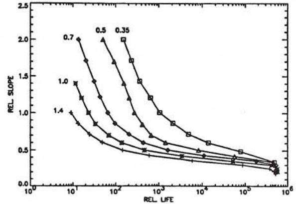
Figure 7 Life reduction caused by dents as a function of the relative slope ( $f_Z/f_X$ ) for different values of  $f_X$ ,  $p_h = 2.5$  GPa,  $b = 0.25$  mm, smooth contact life is  $0.4802 \cdot 10^6$ .
