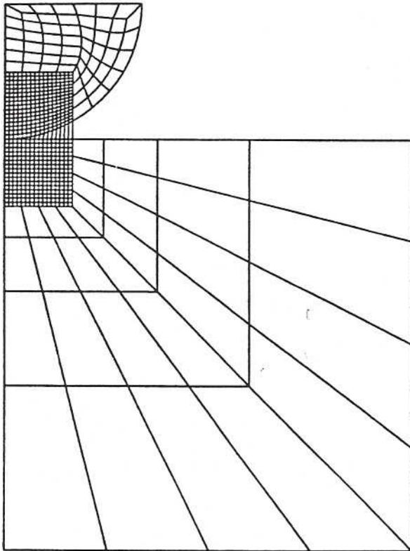
Figure 1 FEM mesh used in indentation calculation.
