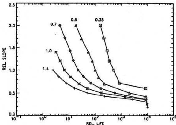
Figure 6 Life reduction caused by dents as a function of the relative slope ( $f_Z/f_X$ ) for different values of  $f_X$ ,  $p_h = 3.0$  GPa,  $b = 0.30$  mm, smooth contact life is  $0.8513 \cdot 10^4$ .
