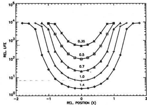
**Figure 5** Life reduction as a function of the dent position relative to the centre of the contact, for a set of dents ( $f_x = f_z = 0.35, 0.50, 0.70, 1.0, 1.4$ ). Contact conditions:  $p_h = 3.0$  GPa,  $b = 0.3$  mm, smooth contact life =  $0.8513 \cdot 10^4$ .
