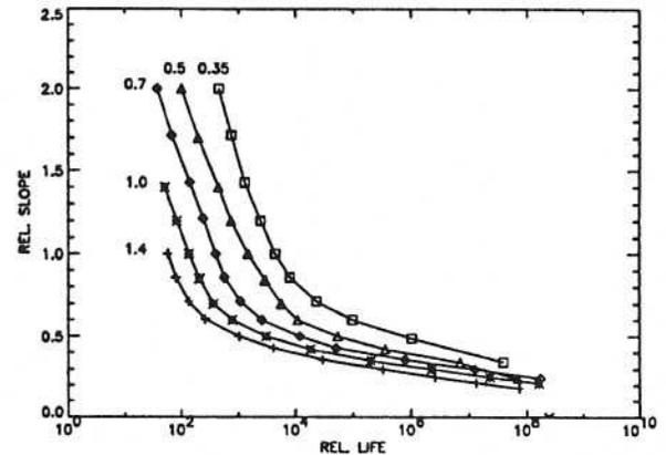
Figure 8 Life reduction caused by dents as a function of the relative slope ( $f_Z/f_X$ ) for different values of  $f_X$ ,  $p_h = 2.0$  GPa,  $b = 0.20$  mm, smooth contact life is  $0.2459 \cdot 10^9$ .
