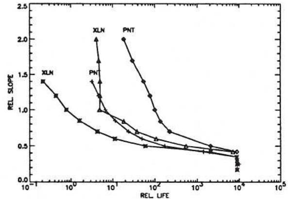
**Figure 3** Comparison of life reductions from the extended line contact analysis with full point contact calculations for two dents,  $f_X = 0.50$  and  $f_X = 1.0$ , as a function of the relative slope  $f_Z/f_X$ .  $p_h = 3.0$  GPa,  $b = 0.3$  mm,  $a/b = 8$ , smooth contact life is  $0.8513 \cdot 10^4$ .
