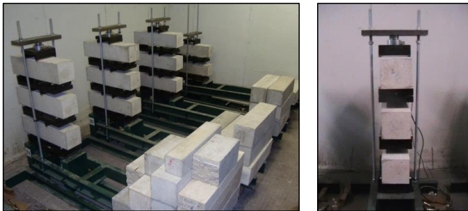
Figure 3. General view of creep test specimens (overview -left- and column detail -right-)
