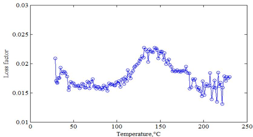
Figure 5: Effects of temperature on loss factor for woven composite material.
