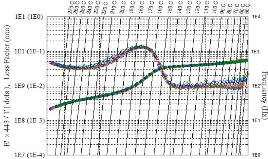
Figure 8: master curves for neat PEEK.
