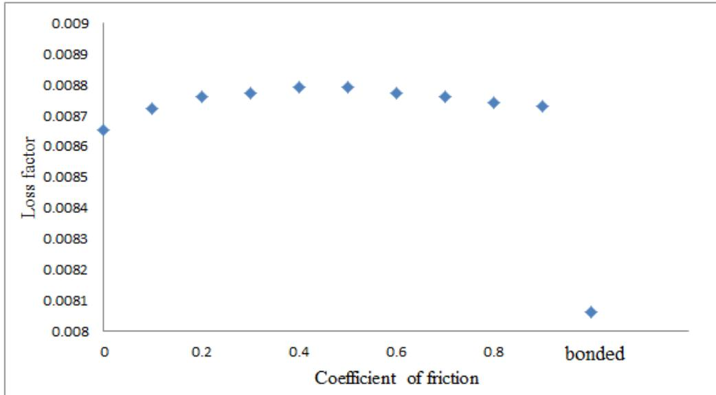
Figure 16: Loss factor at different coefficient of friction.
