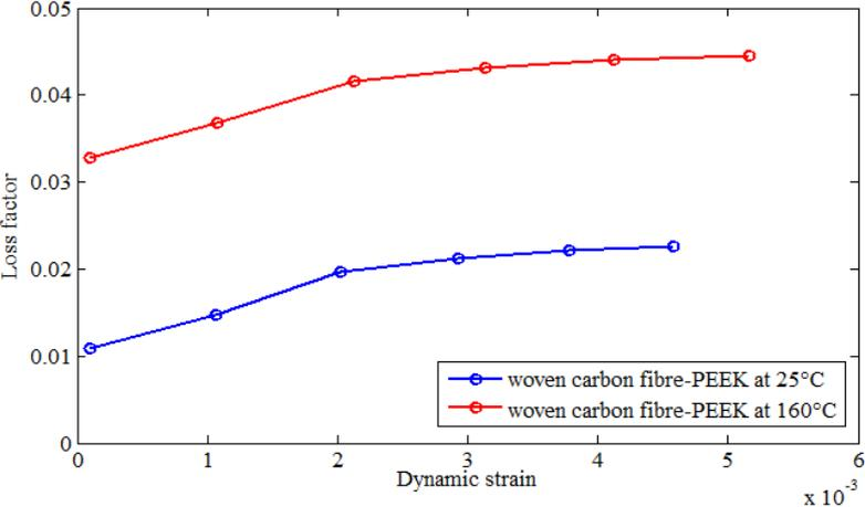
Figure 7: Strain sweep loss factor results for woven composite material.
