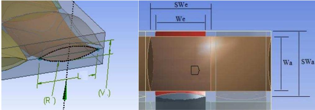
Figure 13: Representative volume element geometry.
