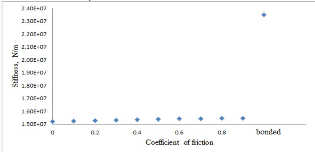
Figure 15: Stiffness at different coefficient of frictions.
