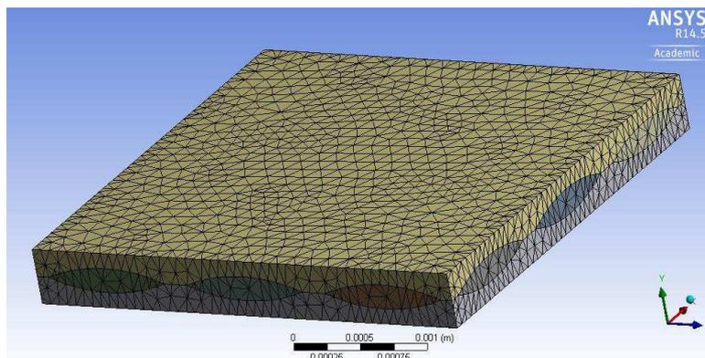
Figure 14: Meshing woven composite unit cell.
