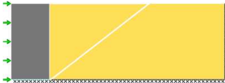
Figure 2: Single wedge failure mechanism for k_h = 0.25 , \delta = \phi = 30^\circ (active force 0.231\gamma H^2 ). Wedge angle is much shallower than static case as expected.
