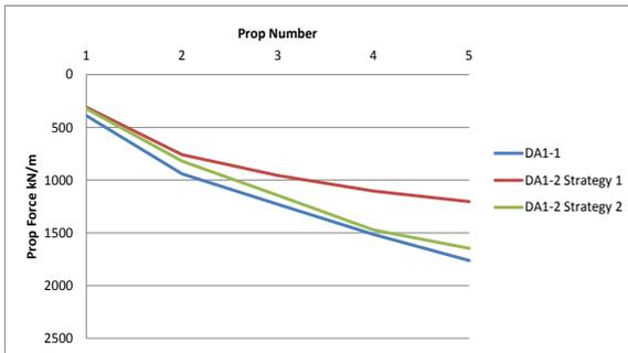
**Figure 4.** Maximum prop loads from different factoring strategies using MC soil model
