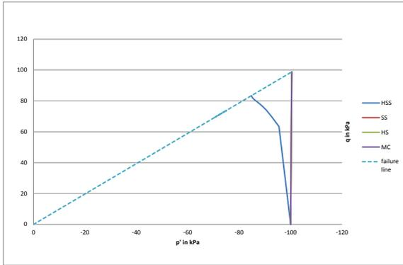
Figure 12. p-q stress paths using different soil models
