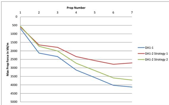
**Figure 8.** Maximum prop loads from different factoring strategies using MC soil model
