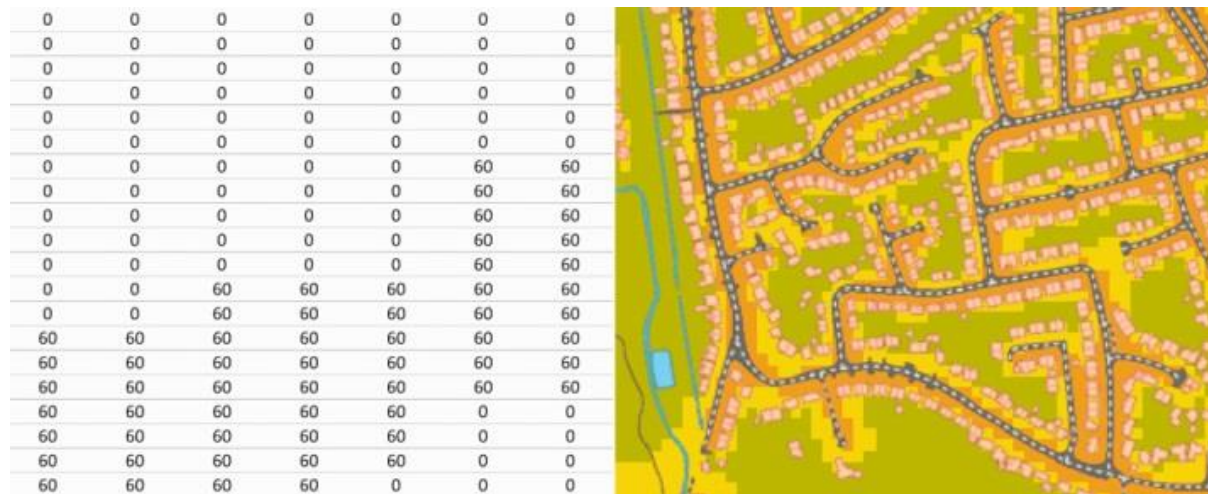
Fig. 5. Matlab code results presenting the transformation from RGB pixel values in dB(A) levels.
