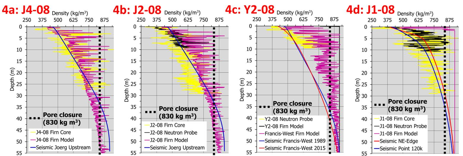
Comparison of depth-density profiles from seismic and borehole (gravimetric firn core analysis, neutron probe) data (note that seismic and borehole acquisitions are not precisely co-located), with simulations from the 1-D firn model.
