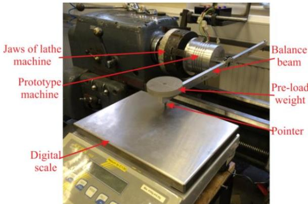
Fig. 16 Test rig for static torque measurements.
