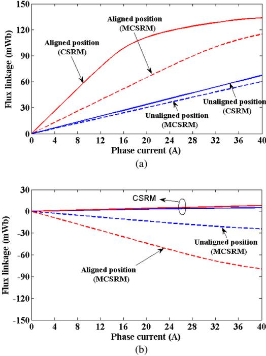
Fig. 3 Self and mutual flux linkages vs phase current for different rotor positions of CSRSM and MCSRM. The phase A supplied by dc current and the mutual flux linkage is captured by phase B. (a) self flux linkage, (b) mutual flux linkages.
