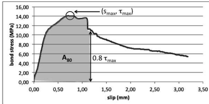
Figure 3: An example of bond stress - slip curve.
