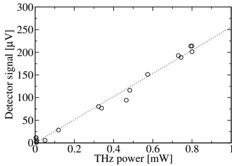
Figure 3. Time-averaged detector response at 2.2 THz as a function of the time-averaged THz QCL power.
