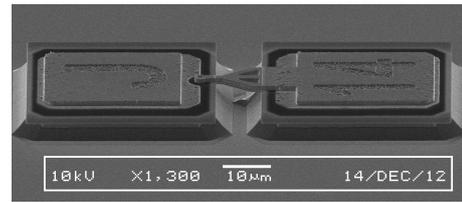
Figure 1. A scanning electron microscope image of a planar airbridged GaAs Schottky diode similar to the devices used in this work
