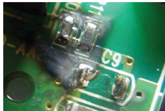
Figure 3. IEMI Damage resulting in the destruction of a surface mount capacitor (Image courtesy of Metatech Corp).
