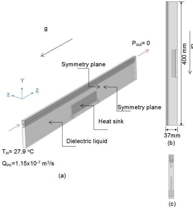
Fig 7. The geometry of the symmetry simulation model used in COMSOL a) Isometric view b) Side view c) Front View
