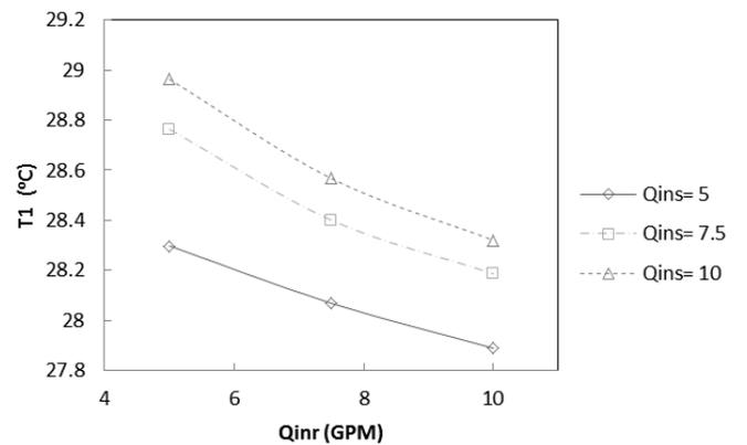
Fig 6. : Water inlet temperature of rack,  $T_1$ , varying  $Q_{inr}$  for different  $Q_{ins}$ .
