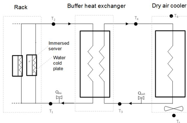
Fig. 1 Schematic diagram of the data center cooling system
