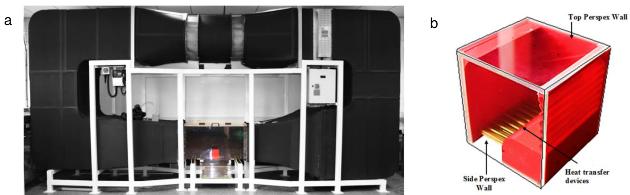
Fig.4 (a) closed-loop wind tunnel (b) 3D printed wind catcher model.
