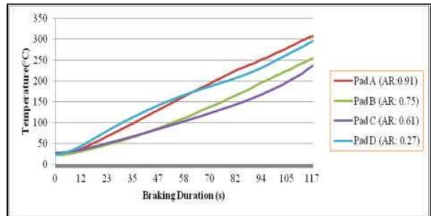
(f) High speed-Med pressure (925 rpm, 2.5 b)
