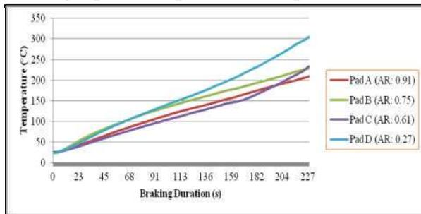
(e) Med speed-Med pressure (545 rpm, 2.5 b)
