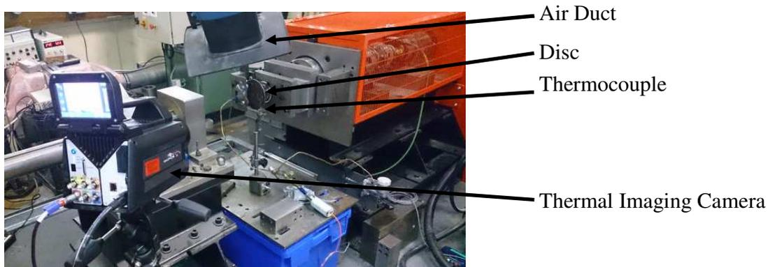
Figure 2: Full Scale Brake Dynamometer Test Rig.
