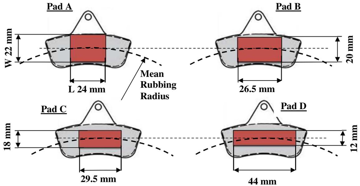
Figure 1: Brake Pads with Different Aspect Ratios (edited [9]).
