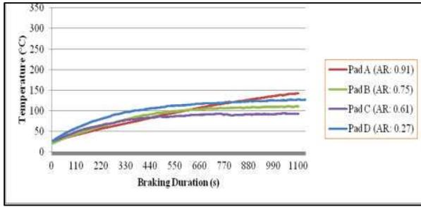
(a) Low speed-Low pressure (185 rpm, 1.5 b)
