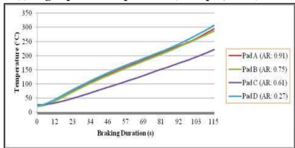
(h) Med speed-High pressure (545 rpm, 4.5 b)
