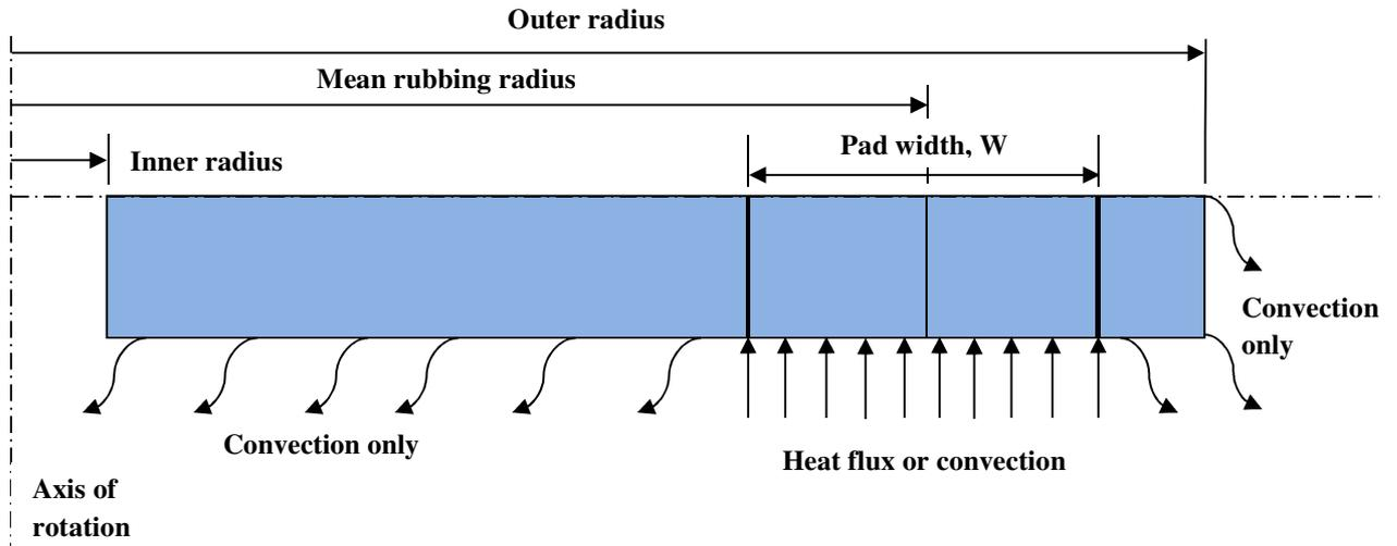
**Figure 4 Outline of finite element model.**
