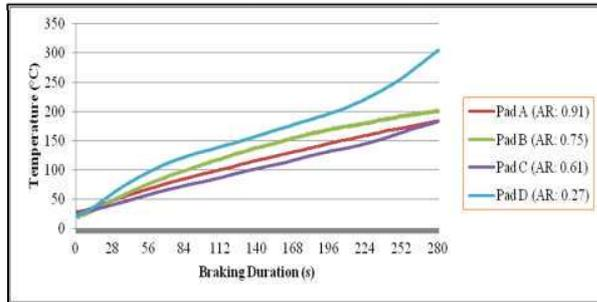
(c) High speed-Low pressure (925 rpm, 1.5 b)
