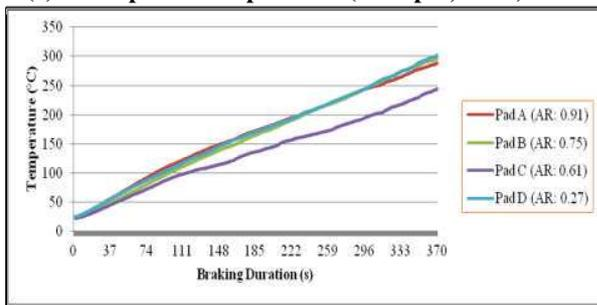
(g) Low speed-High pressure (185 rpm, 4.5 b)
