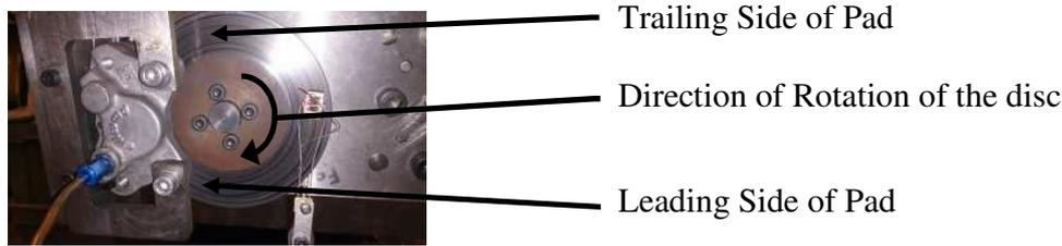
**Figure 3: Position of Thermocouple on the disc.**
