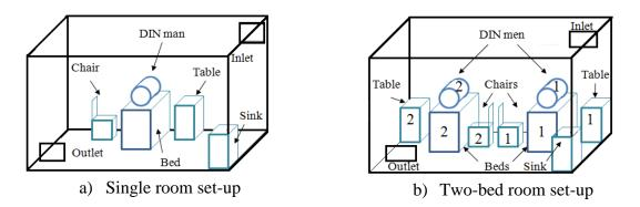
Figure 1. Drawings of room set-up representing hospital single and two-bed rooms (both  $2.26m \ge 3.36m \ge 4.2m$ )
