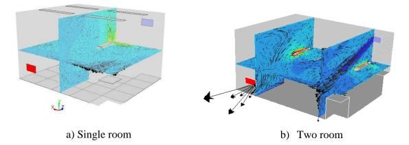
Figure 2. Velocity vectors (0.001-0.1m/s) superimposed over temperature contours (22-37°C)
