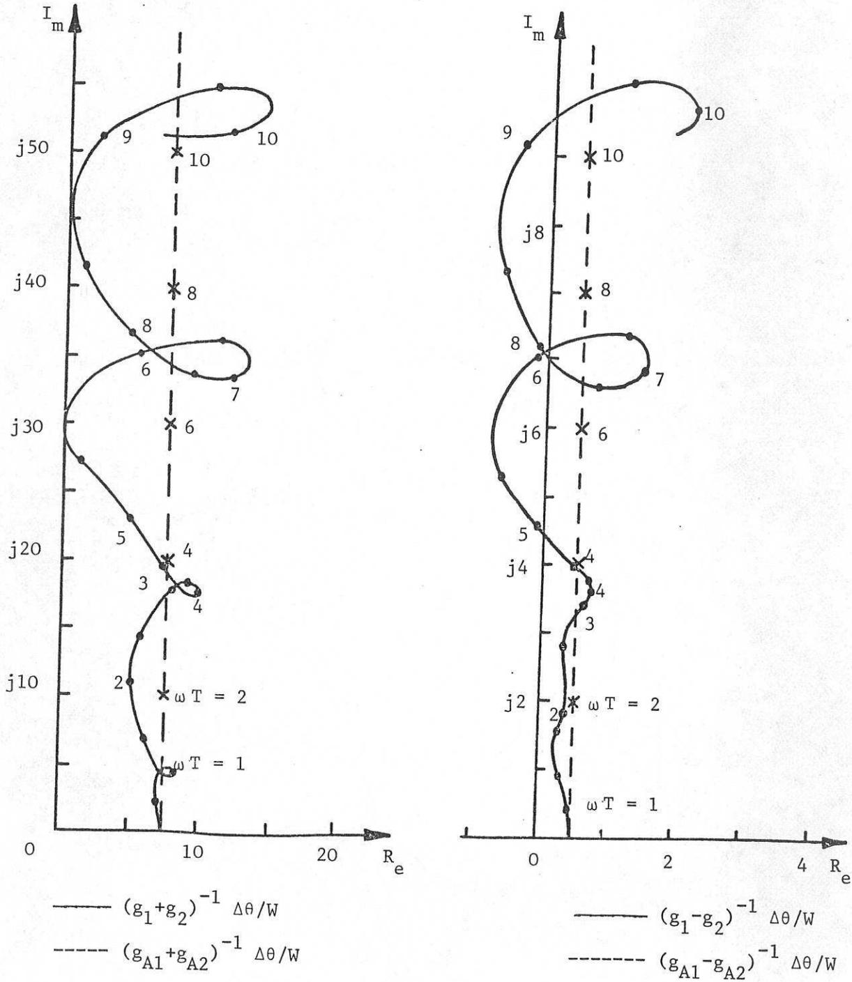
Fig. 5: Inverse Nyquist loci  $c_1^{-1}(j\omega)$  and  $c_{AI}^{-1}(j\omega)$
