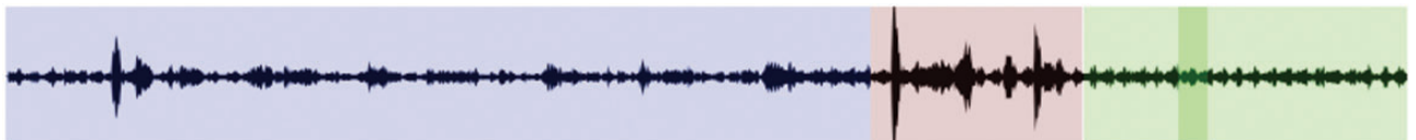
Figure 7. Annotated waveform generated using the Regions plugin for wavesurfer.js. Annotated regions are colour coded by the type of annotation (blue for voice introductions, red for extraneous noise and green for calls). From: http://bio.acousti.ca/node/11778 .
