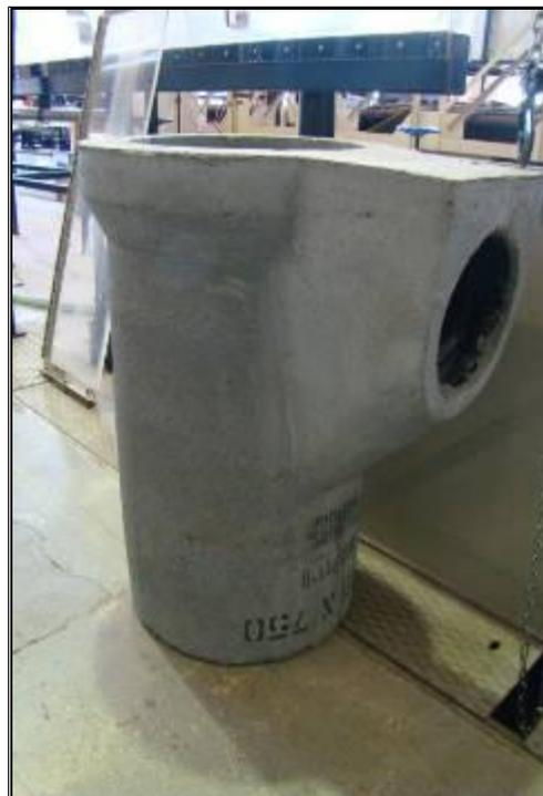
**Figure A2.4: Trapped gully with 150mm diameter outlet**
