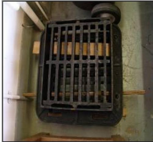
**Figure A2.8: Grate with 325mm x 437mm clear opening (HA102 Reference – S)**
