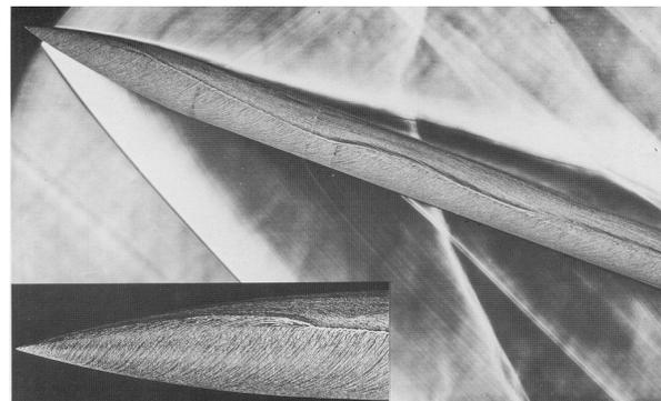
**a) Experimental composite Schlieren/Oil flow photograph**
