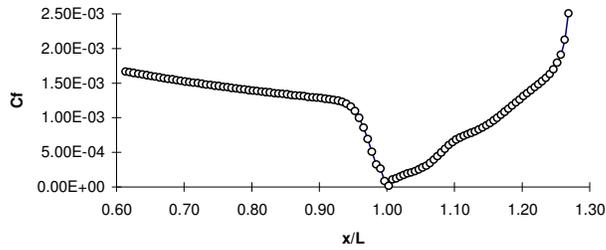
Figure 10: Skin Friction Coefficient Distribution at Incipient Condition
