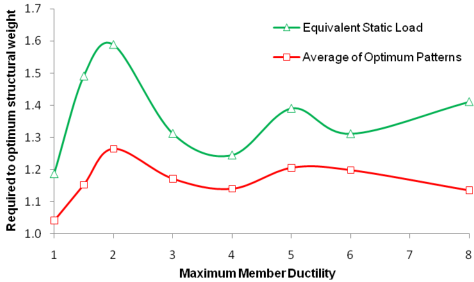
Figure 11. The ratio of required to optimum structural weight for truss structures designed using equivalent static loads and average of optimum material distribution patterns (average for 4 earthquakes)
