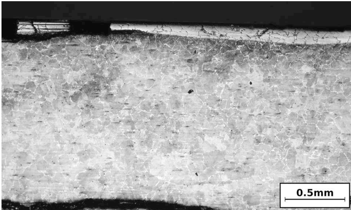
Figure 6 Detail of white etching layer in Figure 5, rail UC10010. Thickness of the layer is approximately 125\mu\text{m} at its deepest point. The microstructure shows very little plastic flow, either at the surface, or on the boundary of the crack at the bottom of the figure. The ferrite of the original microstructure remains visible inside the white etching layer.
