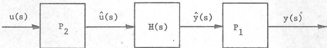
Fig. 2 Dyadic Decomposition of the Plant G(s)
