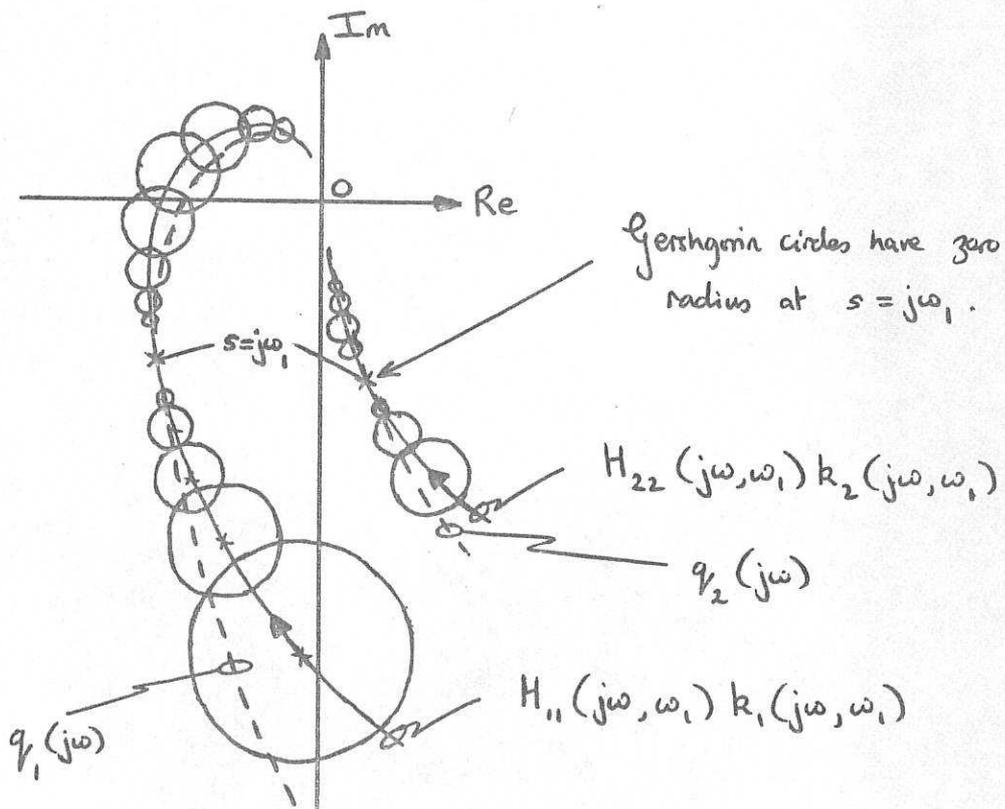
Fig. 7 Schematic Representation of Rational Approximation
