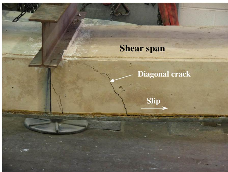
Figure 5: Shear crack and longitudinal slip near the shear span
