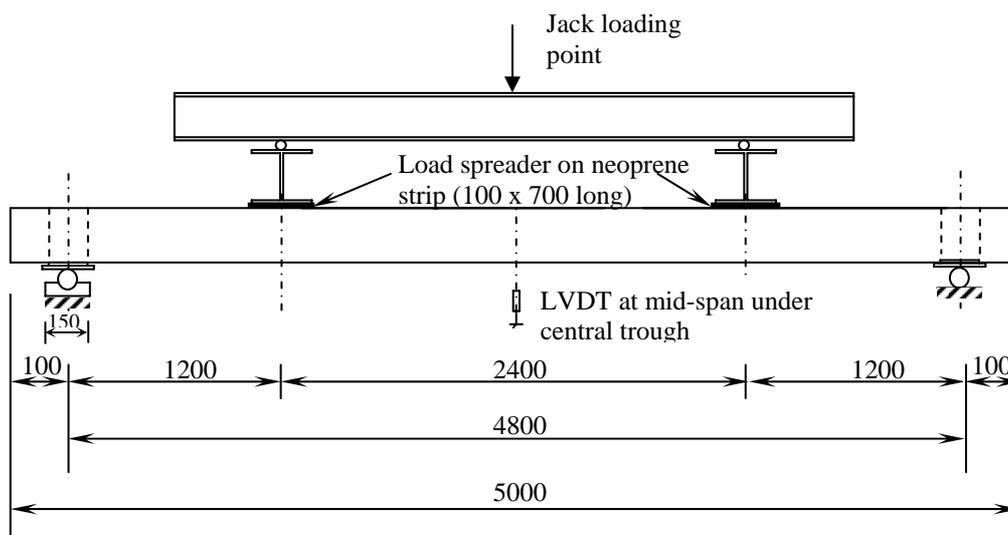
Figure 1: Test arrangement for the long-span composite slabs
