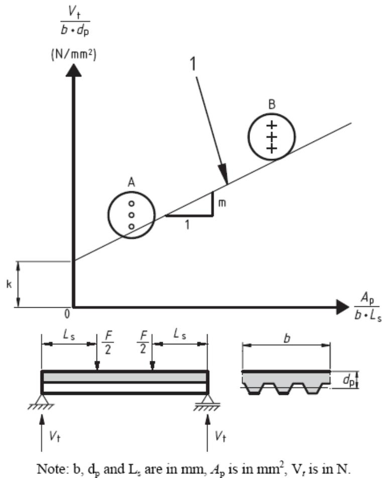
Figure 7: Evaluation of test results (BS EN 1994-1-1:2004 Annex B)
