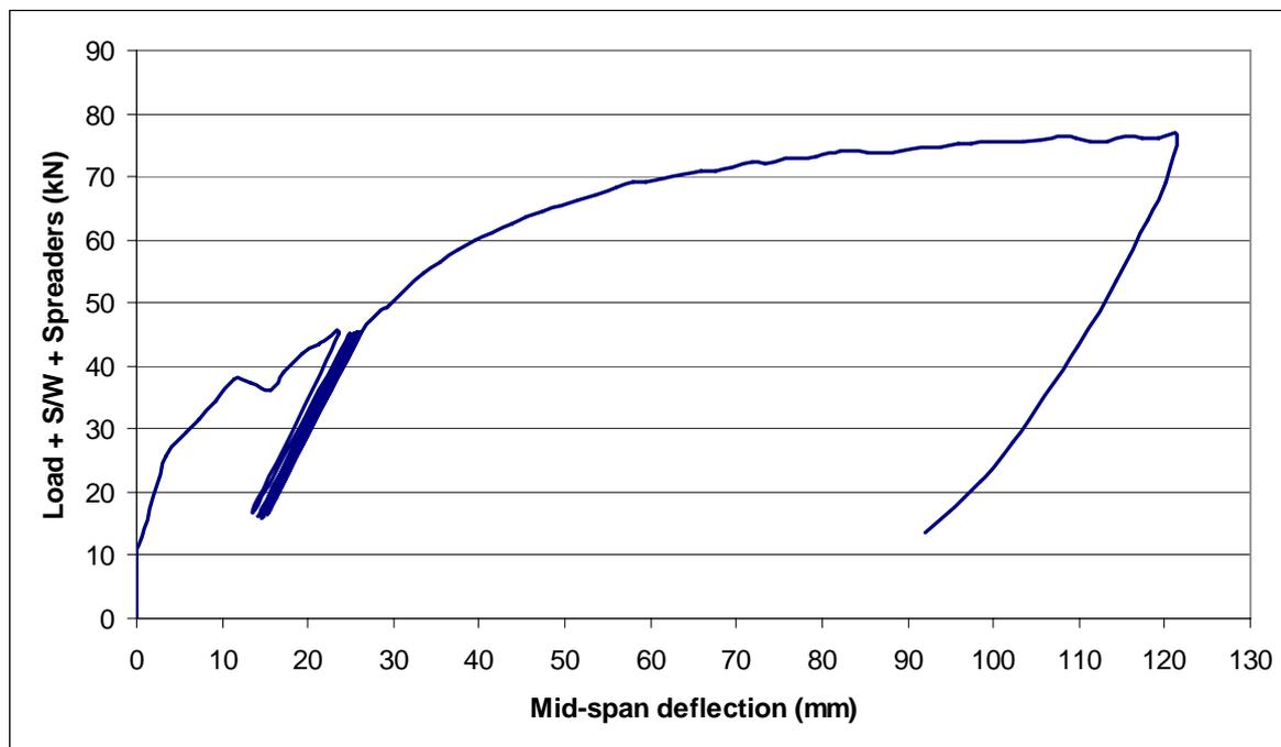
Figure 6: Cyclic test for the long-span specimen
