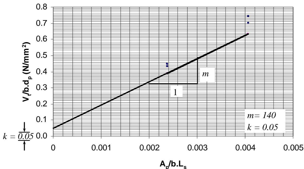
Figure 8: The  $m$ - $k$  curve for composite slab
