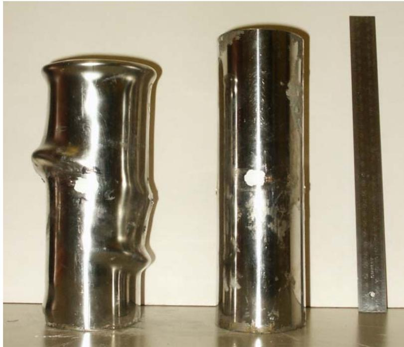
Figure 5: Comparison between tested and untested composite EHS column
