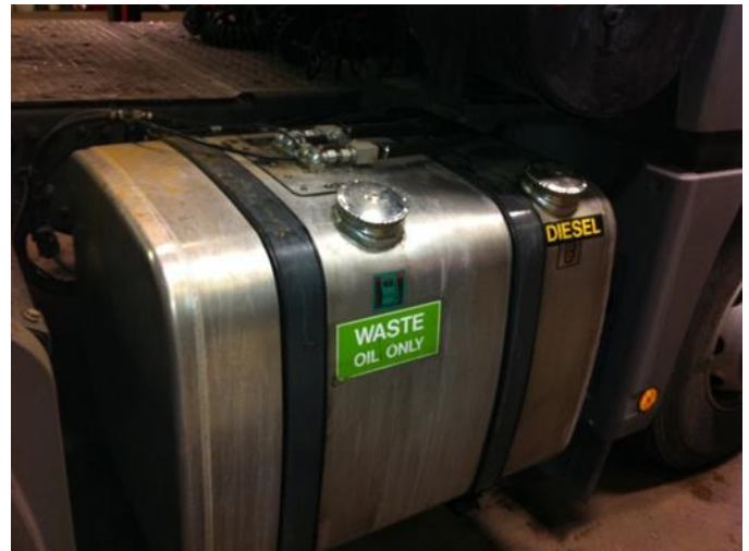
Figure 2: A dual fuel tank in a 44-tonne truck
