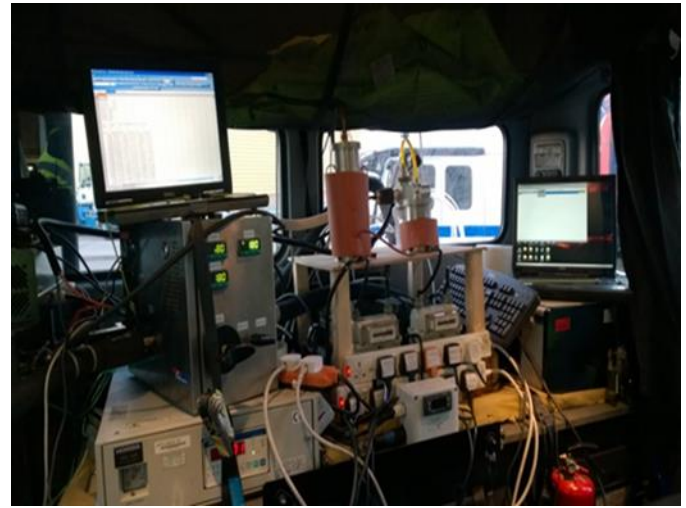
Figure 4: On-board PM and gaseous sampling system
