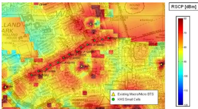
Fig. 6. Simulated macrocell & microcell best server RSCP coverage along KHS following activation of the thirteen +24dBm KHS microcells.
