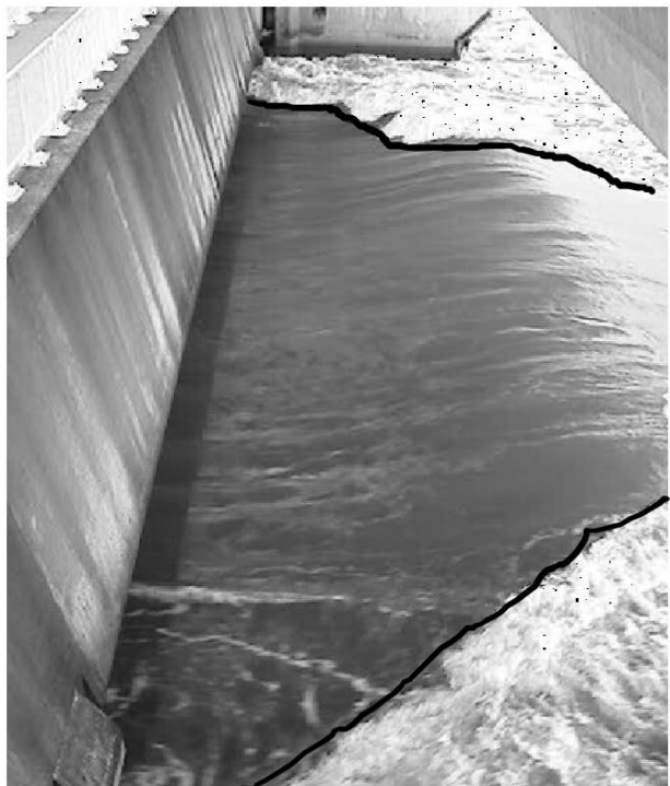
FIG. 1: Examples of (a) one oblique hydraulic jump in a roadside stream flowing into an underpass (picture courtesy Valerie Zwart), top view and flow from right to left; and, (b) two oblique hydraulic jumps in the tidal flow rushing out of one of the sluices in the Oosterschelde storm surge barrier in The Netherlands, side view and flow from left to right. Black lines indicate the hydraulic jumps.
