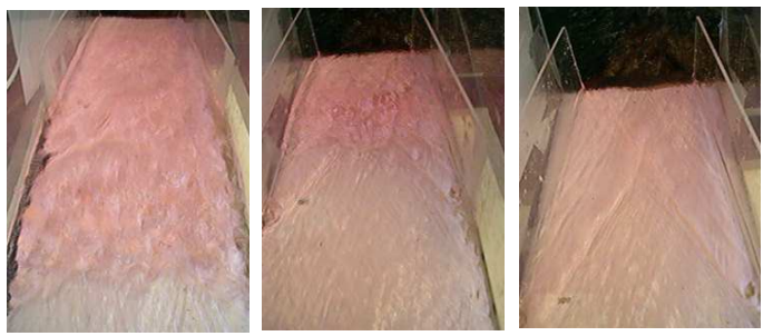
FIG. 8: Multiple states appear for F_0 = 3.07 and B_c = 0.7 , marked by a star in Figure 6. From left to right these states are: an upstream steady shock, the reservoir state, and oblique waves. Each transition is induced by blocking or pushing the flow with a small paddle.
