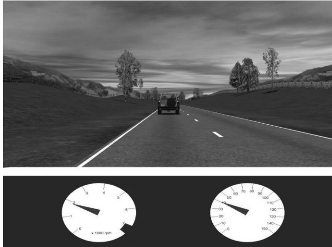
Figure 2. Simulator screenshot showing the participants forward field of view. Speedometer and tachometer functioned realistically
