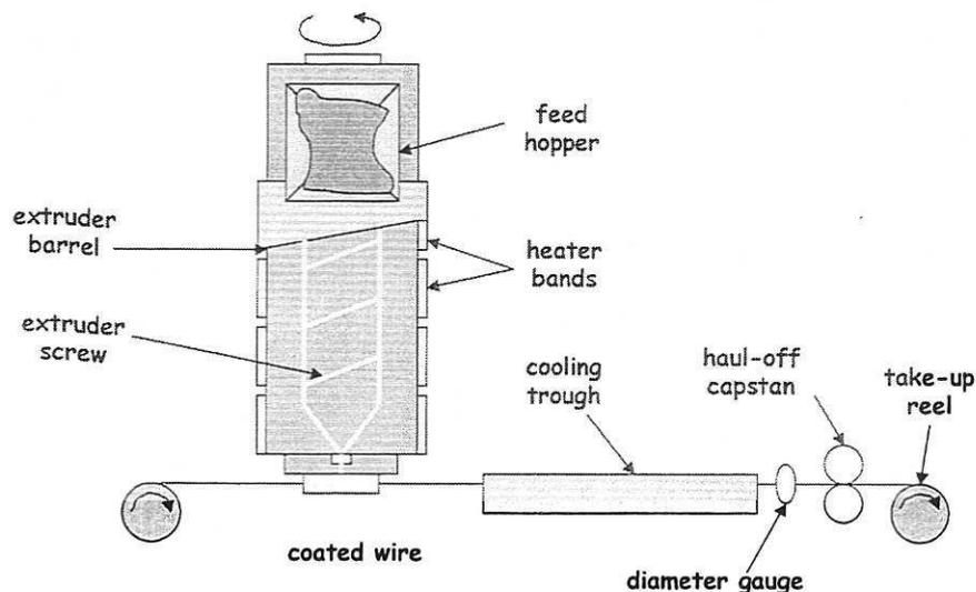
Fig. 2. Cable extrusion process.
