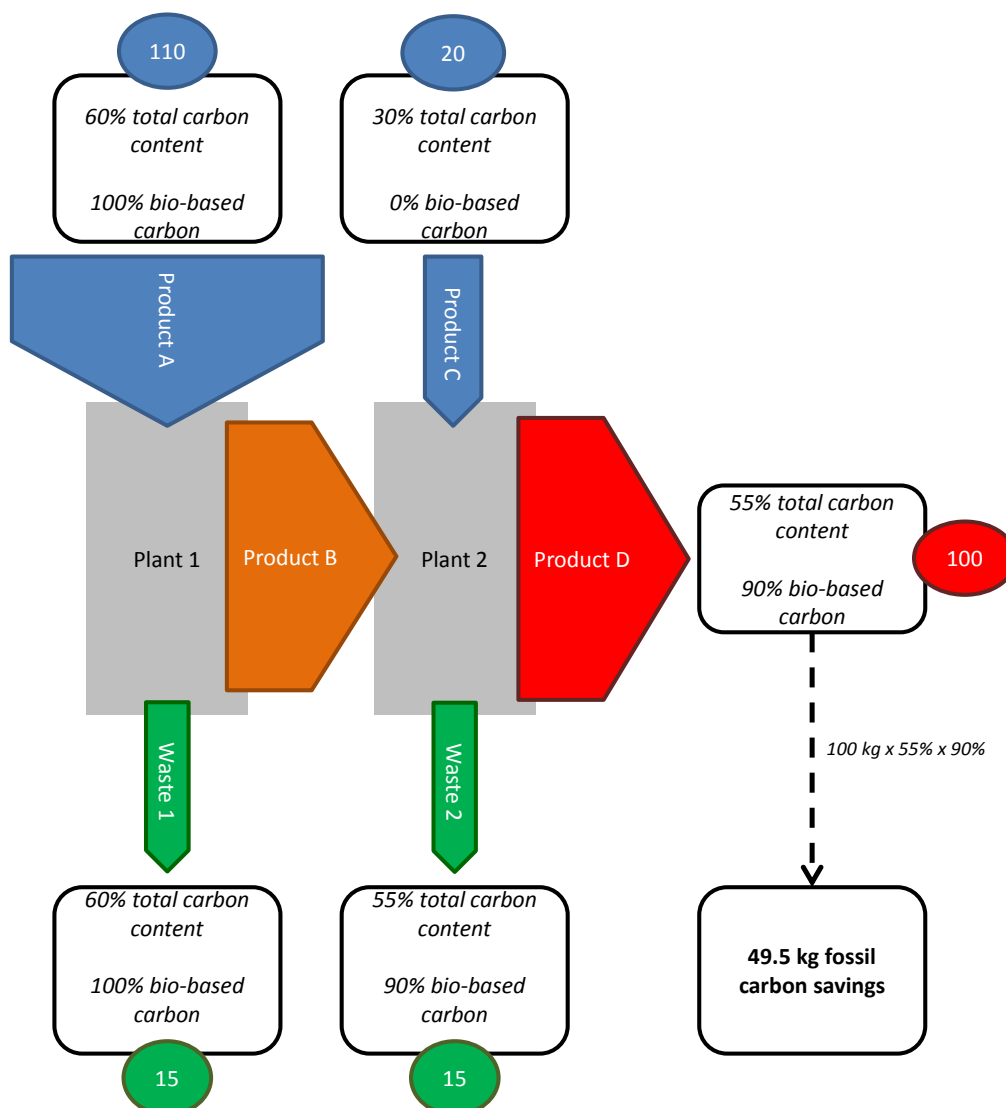
Figure 5-6 Mass balance approach to calculate the amount of bio-based carbon/fossil carbon saved in the global supply chain in a dedicated facility with mass flows described in units of kilograms.
