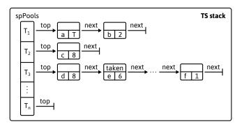
Figure 2: The TS stack data-structure.
