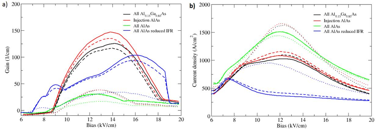
Figure 1: Gain (a) and current (b) versus applied bias for the reference structure [2], reference with AlAs injection barrier and all AlAs barrier structures [3] at 4.2 K (solid), 77 K (dashed) and 200 K (dotted) lattice temperatures.
