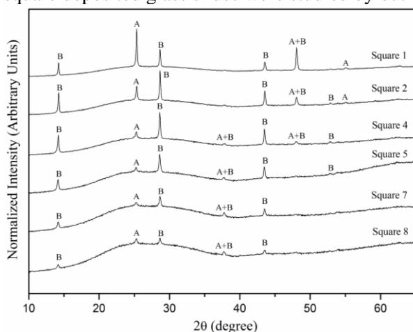
**Figure 1.** Out of plane XRD patterns of TiO<sub>2</sub> thin film prepared by LPCVD at 600°C: A and B refer to the assignment of the anatase and TiO<sub>2</sub>(B) phases respectively.
