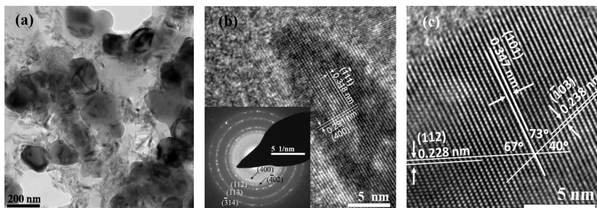
**Figure 5.** (a) A TEM image taken from Square 4, showing both anatase polygonal plates and  $\text{TiO}_2(\text{B})$  needle-shaped particles; (b) HRTEM of a  $\text{TiO}_2(\text{B})$  needle and SADP of a group of the needles; (c) HRTEM image of an anatase polygonal plate.
