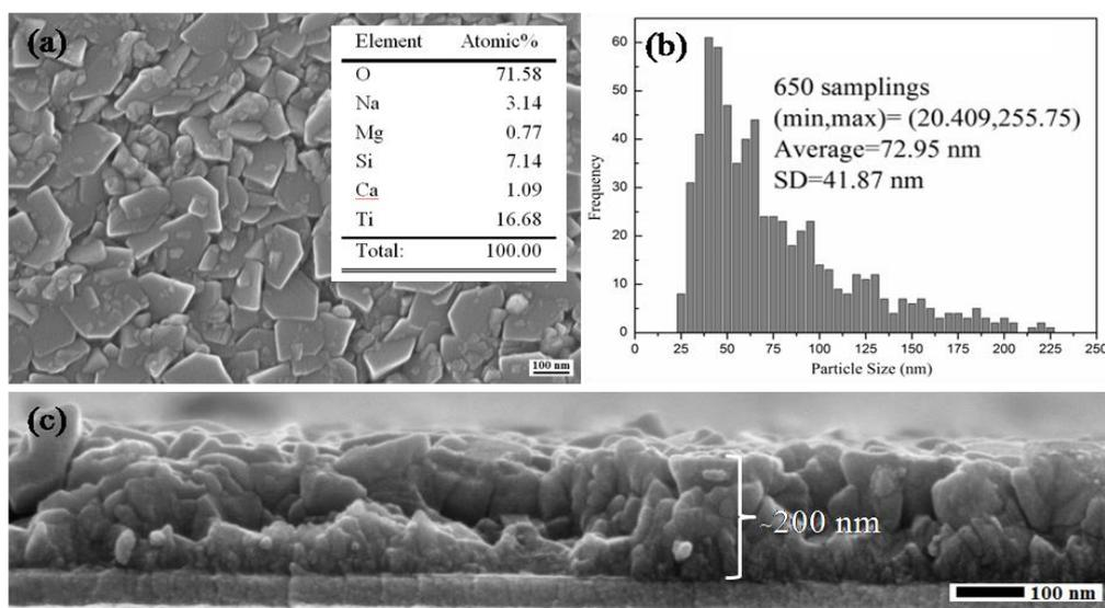
**Figure 4.** (a) SEM secondary electron image of TiO<sub>2</sub> thin film from Square 4; (b) Primary Particle Size Distribution measured from measurement of 650 particles; (c) SEM cross-sectional image of thin film thickness after fracturing the glass slide.
