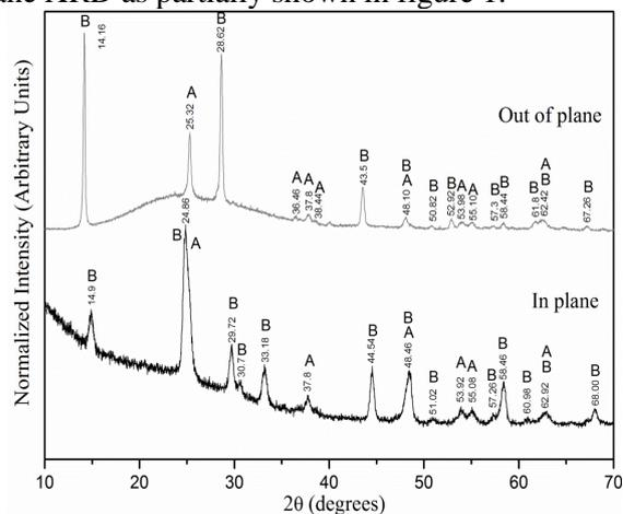
**Figure 2.** In plane and out of plane XRD patterns of Square 4: A and B refer to anatase and TiO<sub>2</sub>(B) phases respectively.
