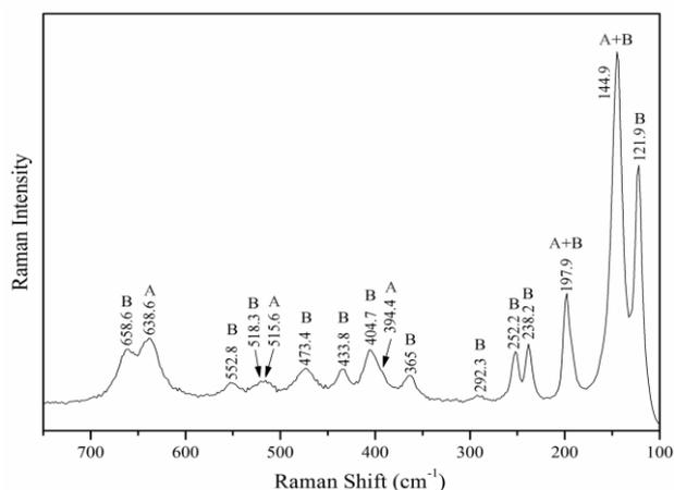
**Figure 3.** Raman spectrum of Square 4: A and B indicates the anatase and TiO<sub>2</sub>(B) phases respectively.
