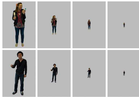
Figure 3 Example of target people at the four different sizes representing four observation distances. At full size these were printed on A3 paper.
