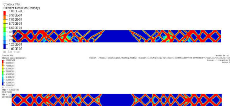
Figure 7 - a) Results of a topology optimisation study on a beam web; b) Results of a topology optimisation study on a beam web incorporating a symmetry constraint
