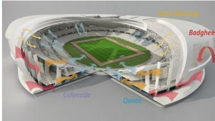
Fig. 4 Evaporative cooling technique suggestion for 2022 World Cup stadiums [33].
