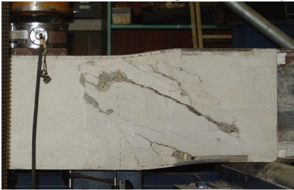
Fig. 15: USFB No.3 (concrete bursting)
