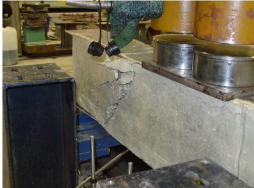
Fig. 14: USFB No.2 (concrete bursting)
