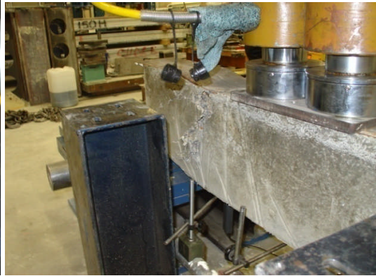
Fig. 13: USFB No.1 (concrete bursting)
