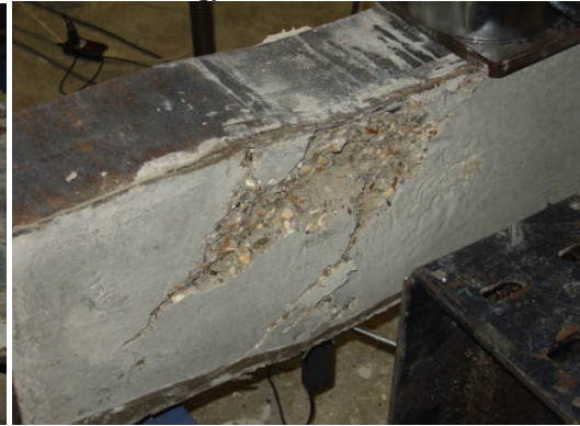
Fig. 15: USFB No.3 (concrete bursting)
