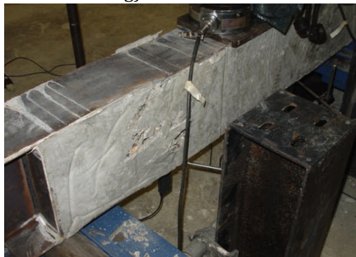
Fig. 16: USFB No.4 (concrete bursting)
