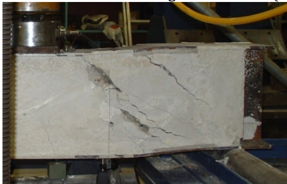
Fig. 16: USFB No.4 (concrete bursting)
