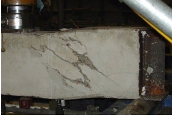
Fig. 13: USFB No.1 (concrete bursting)
