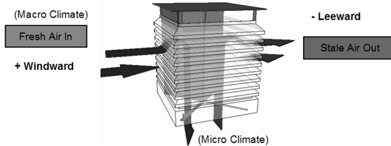
Figure 1: A flow diagram representing ventilation through a multi-direction wind tower
