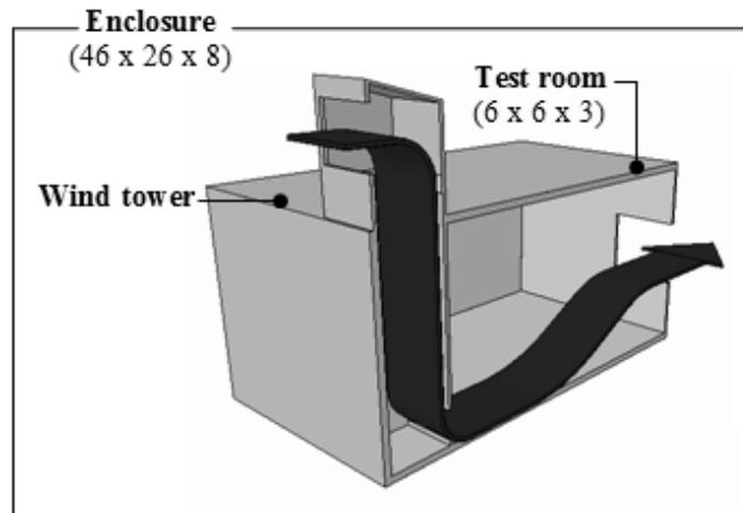
Figure 3: Schematic of a wind tower system mounted on the test room
