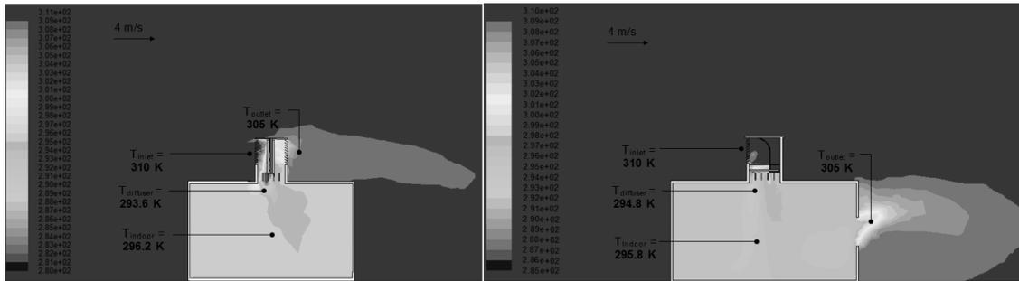
Figure 8: Temperature distributions inside the test room with a commercial wind tower incorporating the vertical HTD arrangement (a) and horizontal HTD arrangement (b).
