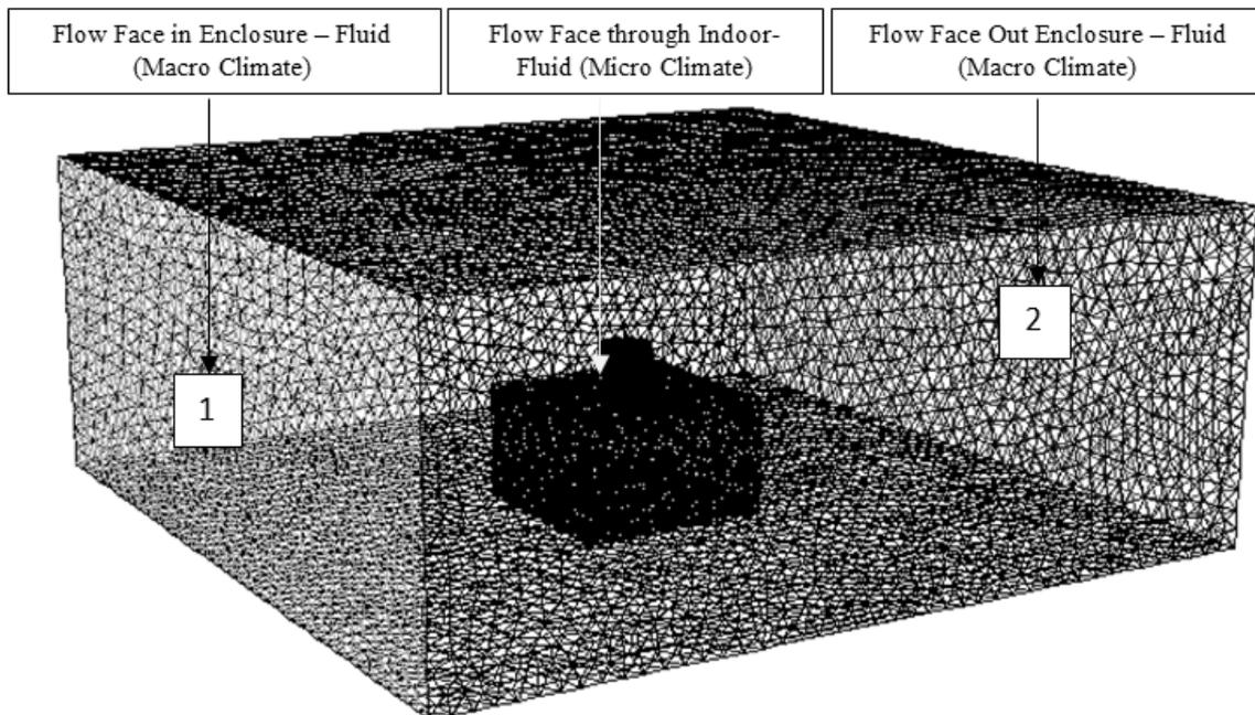
Figure 4: Flow domain representation of the physical geometry of the wind tower design under investigation and location of set boundary conditions
