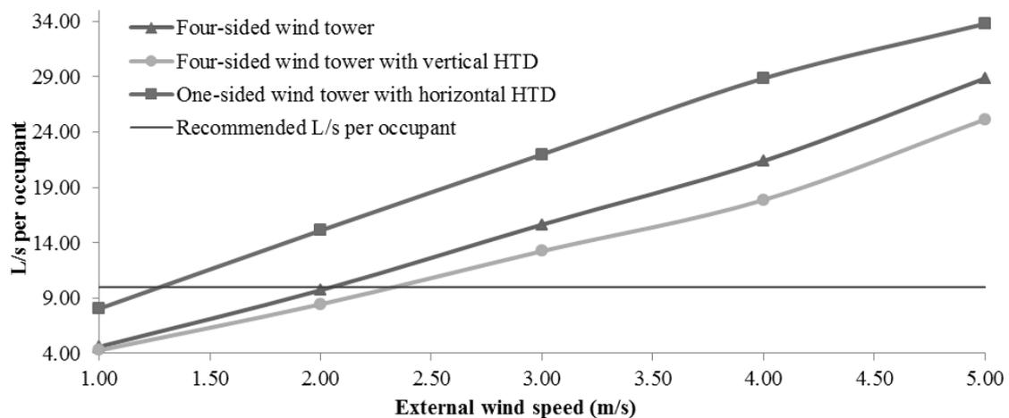
Figure 7: Comparison of the air supply rates of the wind tower configurations at various external speeds
