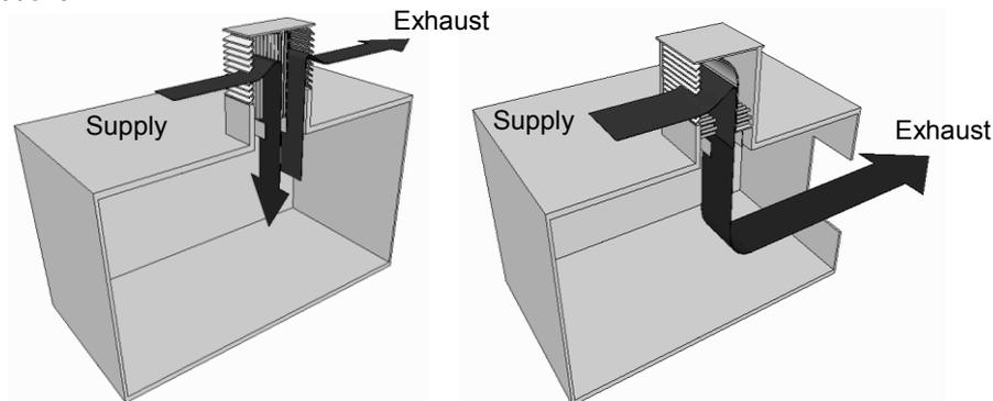
Figure 2: Wind tower systems incorporating (a) vertical HTD arrangement (b) horizontal HTD arrangement
