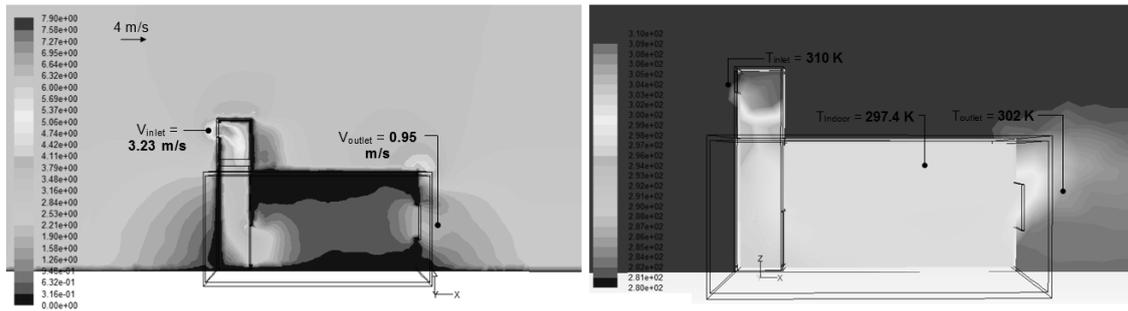
Figure 6: Velocity contour lines of a cross sectional plane in the test room with (a) Temperature distributions within the test room with the evaporative cooling tower (b)
