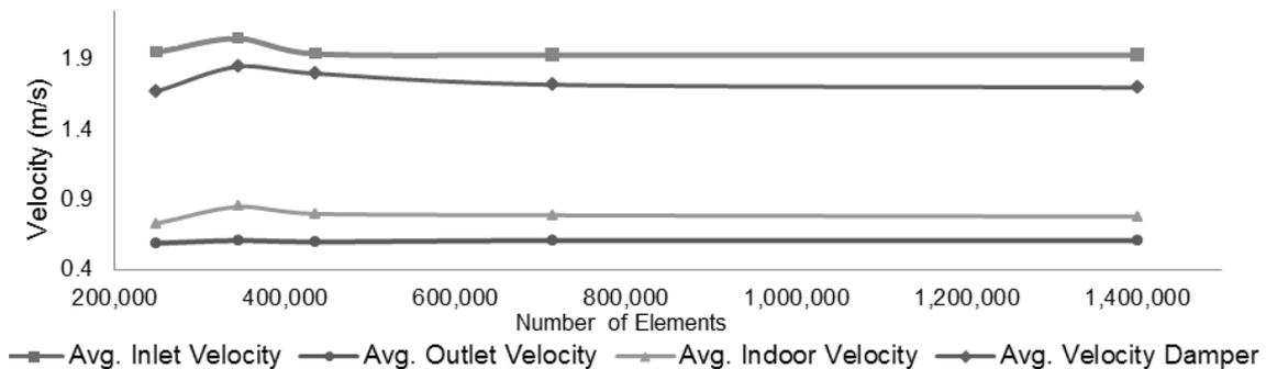
Figure 5: Comparison of solutions from various grid adaptation methods. The variables are the average velocity at the inlet and outlet of the wind towers and interior of the test room
