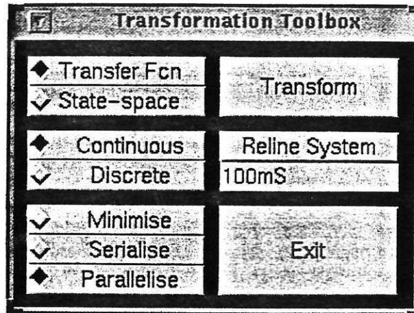
Figure 5: The Transformation Toolbox graphical user interface.
