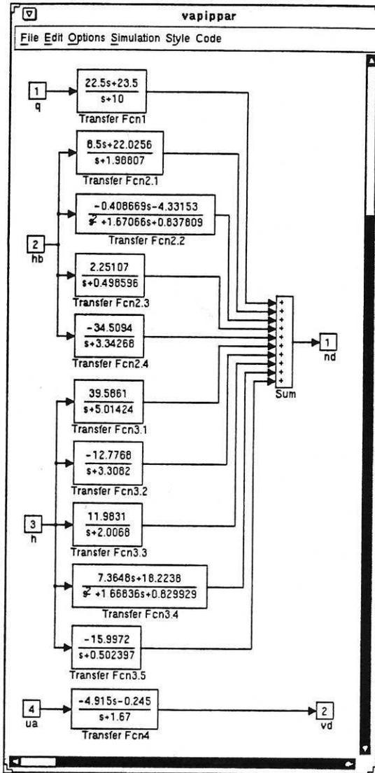
Figure 7: The parallelised independent path representation of the VAP control law.
