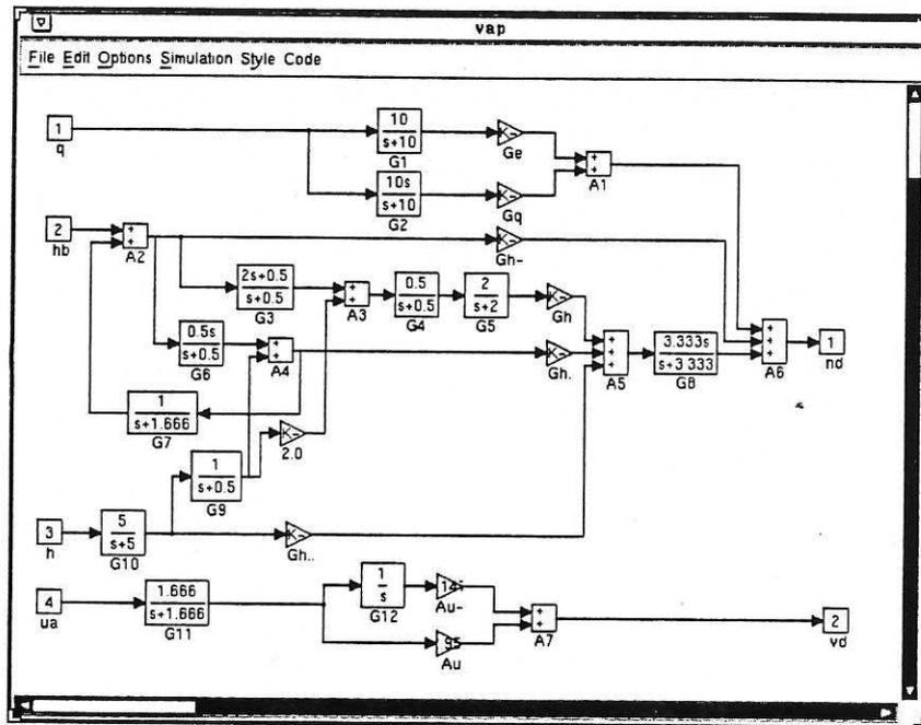
Figure 2: VAP flight control law entered into Simulink
