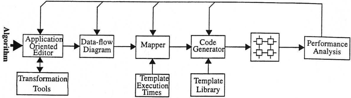
Figure 1: Heterogeneous System Development Cycle
