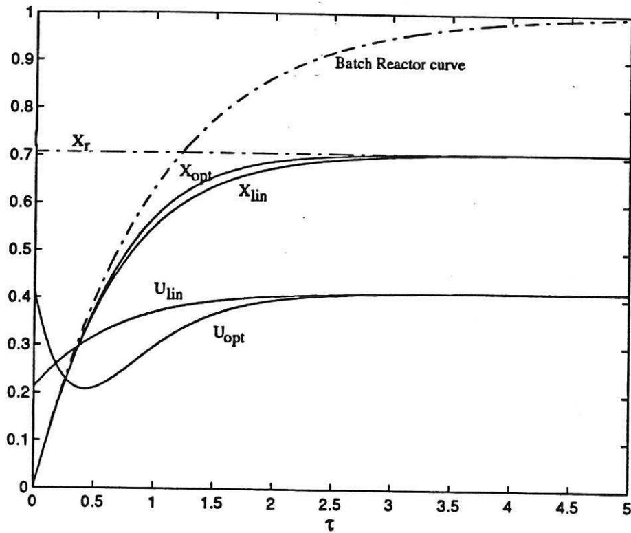
Fig. 7. Comparing the responses of the optimal and linearly controlled process for equal minimum flow conditions.
