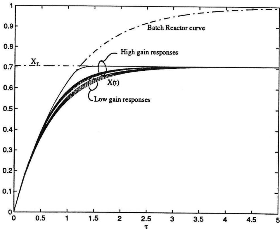
Fig. 4. Comparing high and low gain control responses of  $X(\tau)$  from Fig. 2 and Fig. 3
