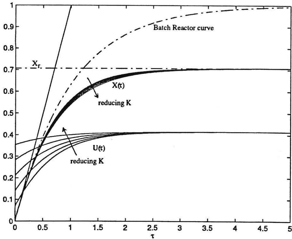
Fig. 2. Responses of CSTR under linear proportional control
