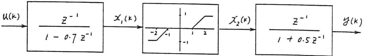
Figure 5.1 Dynamic system with dead zone & saturation
