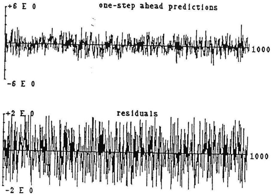
Figure 5.3 One step ahead predictions & residuals for the identified model of the dynamic system with dead zone & saturation
