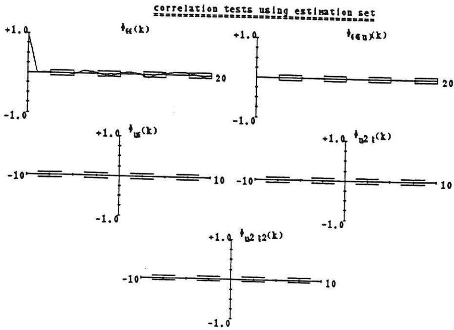
Figure 4.3 Model validation for the exponential time series
