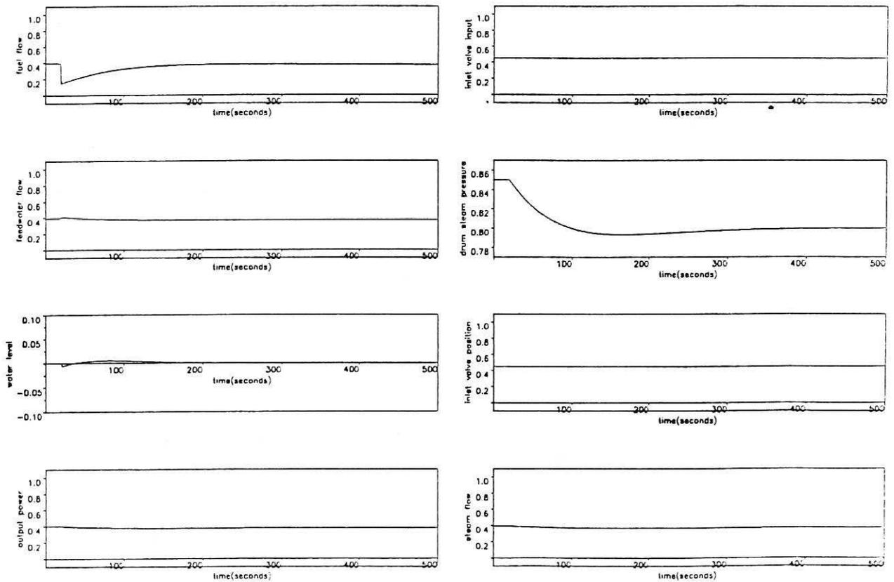
fig. 6: The boiler response to drum steam pressure demand change with two PI regulator
