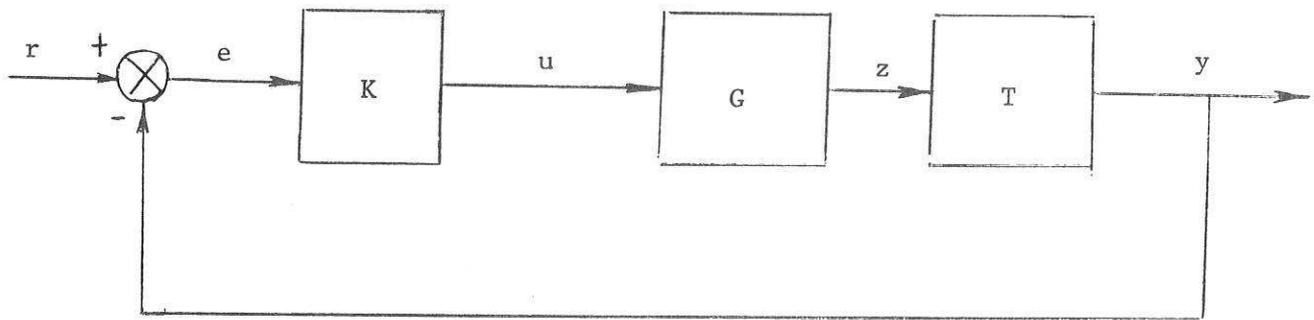
Fig.5. Normal Feedback Control Scheme
