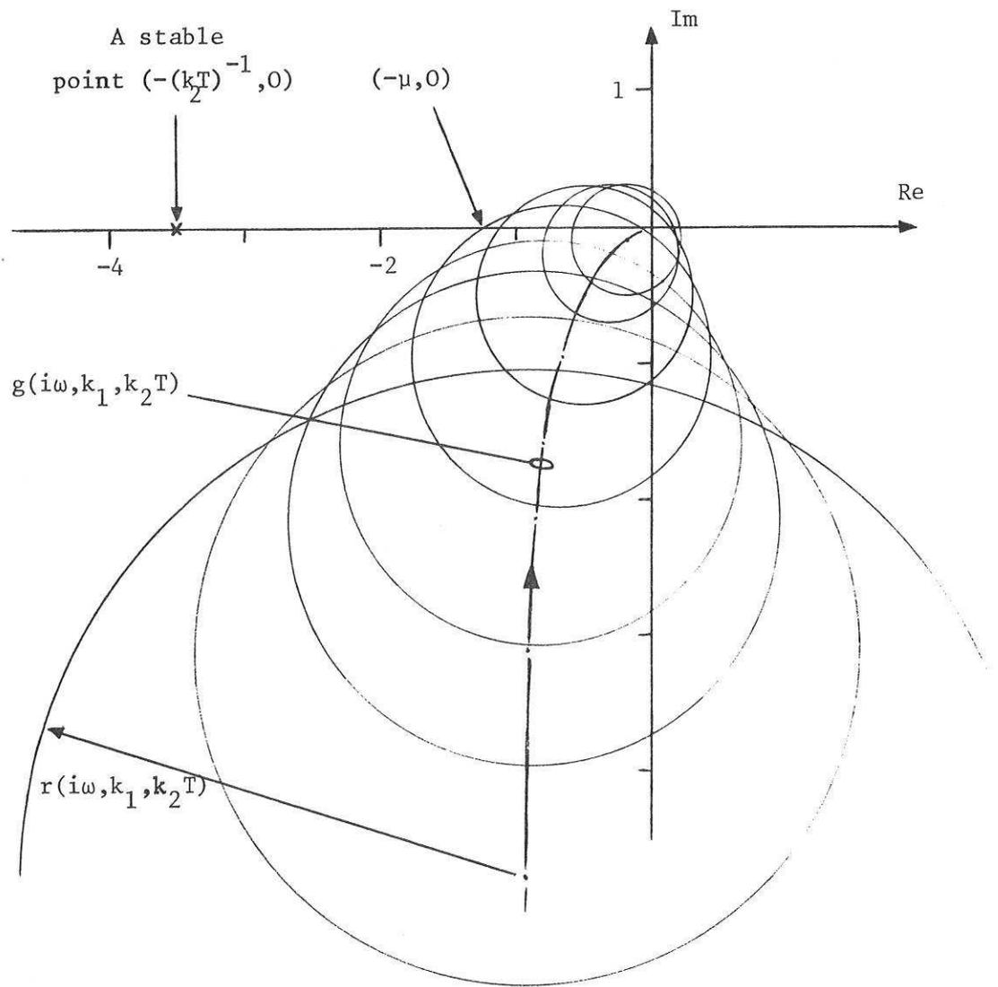
Fig. 1. Graphical Stability Criterion and
