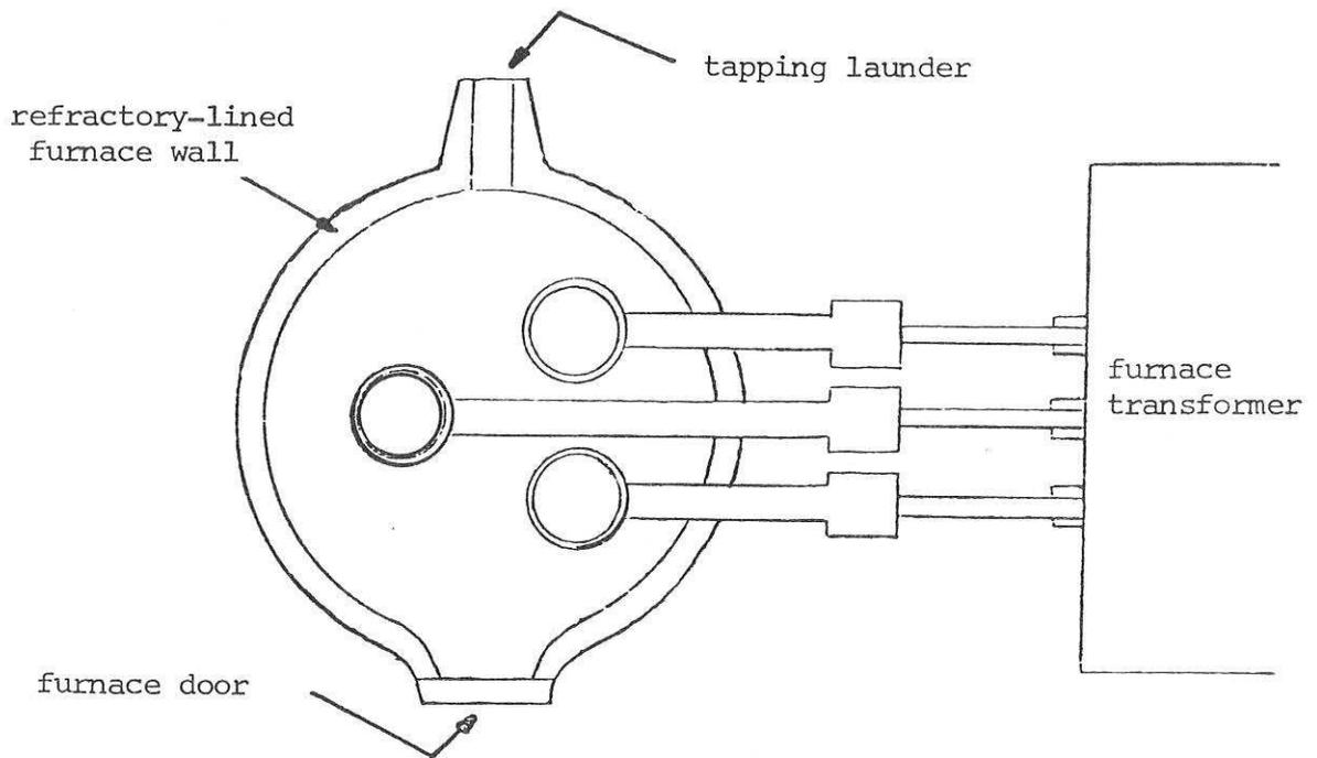
CONSTRUCTION OF ARC FURNACE
