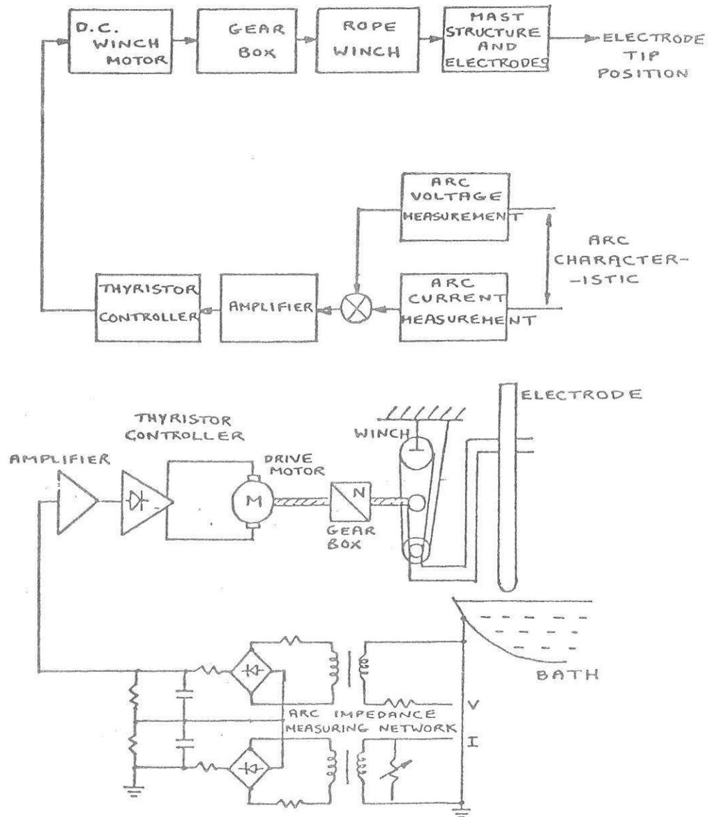
A direct-haul d.c. motor driven electrode position controller
