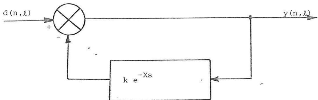
Fig. 4 Automatic steering process block-diagram
