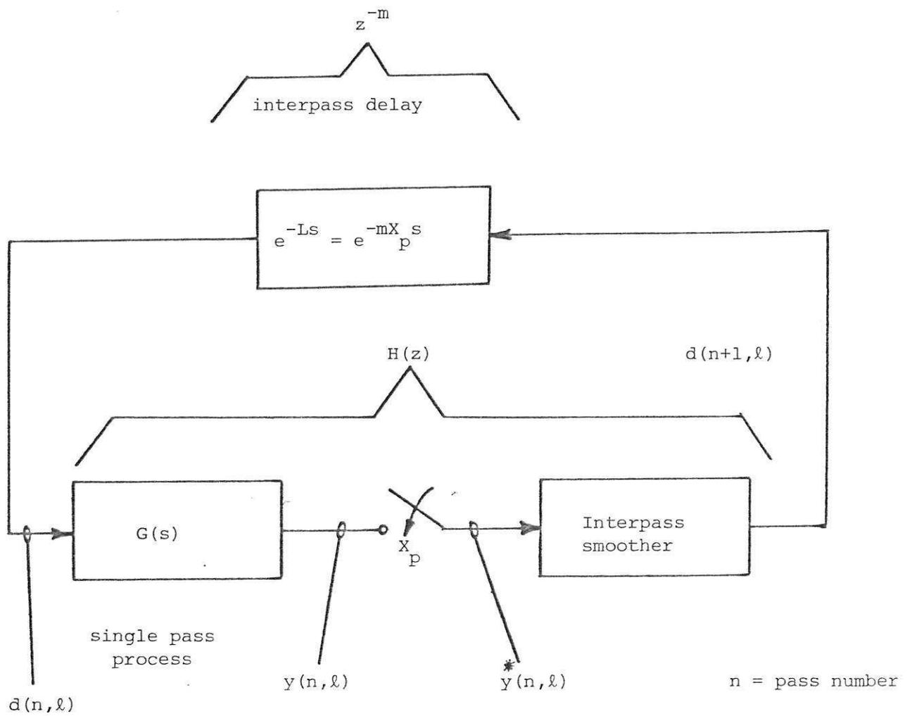
FIG. 1 Multipass process with discrete interpass smoothing
