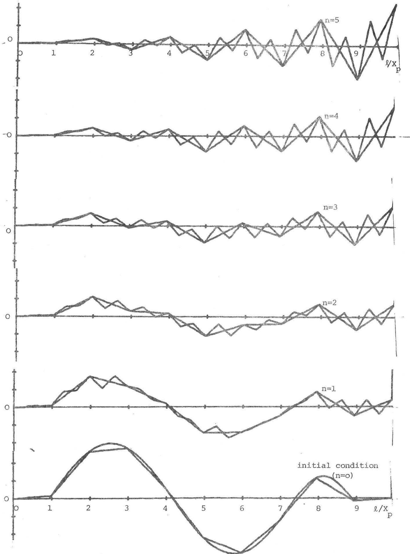
Fig. 10 Traces of  $y(n, \ell)$  and  $d(n+1, \ell)$  showing multipass instability ( $r=3, k = 0.95$ )
