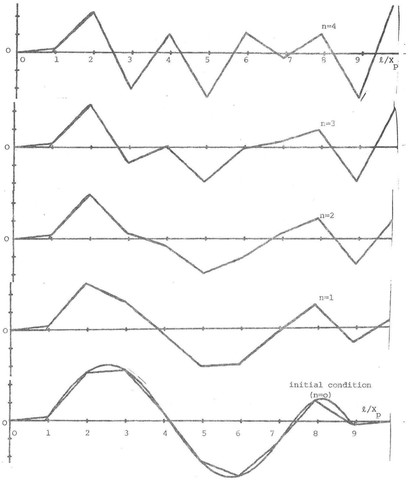
Fig. 9 Traces of  $y(n, l)$  and  $d(n+1, l)$  showing multipass instability
