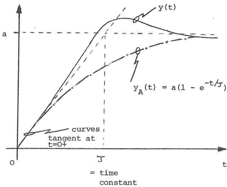
Fig. 2. Construction of Approximate First Order Model from Time Constant and Steady State Data
