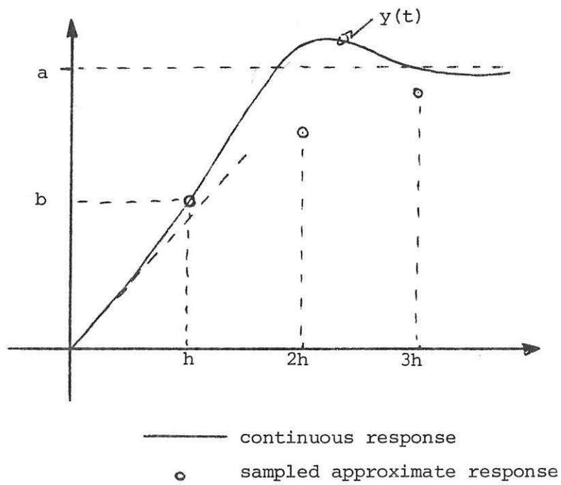
Fig. 4. Graphical Construction for Approximate First-order Discrete System
