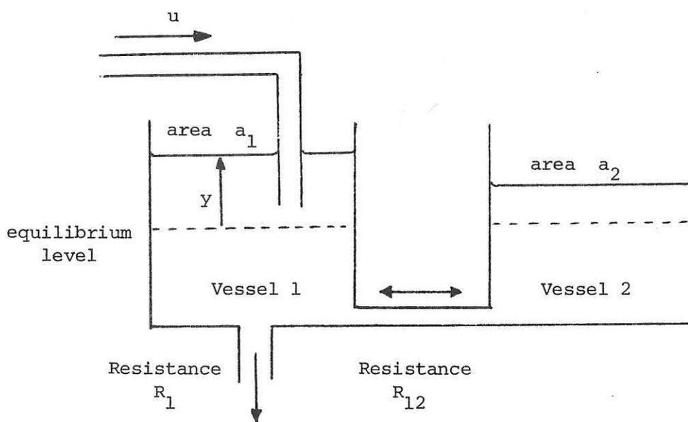
Fig. 5. Liquid Level System
