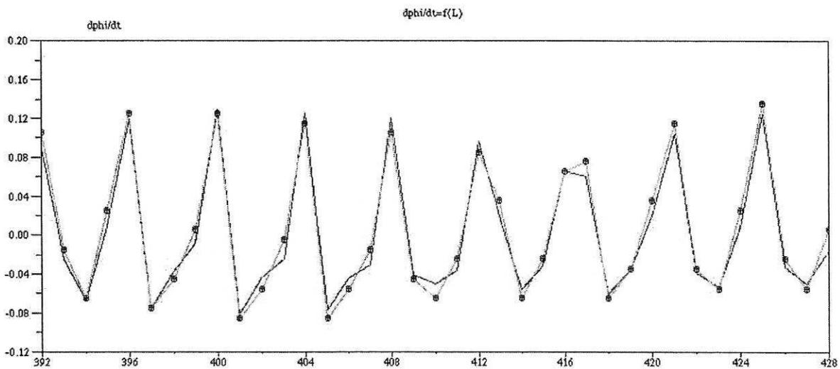
Figure 7: MODELLING THE ROBOT'S MOTOR RESPONSE (ROTATIONAL VELOCITY  $\dot{\phi}$ ) AS A FUNCTION OF LASER SENSOR PERCEPTION  $L$  (SEE ALSO TABLE 2). TRUE ROTATIONAL VELOCITY IS SHOWN AS A SOLID LINE WITH CIRCLES, THE MODEL-PREDICTED OUTPUT AS A SIMPLE SOLID LINE.
