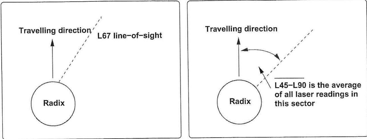
Figure 5: L67 (MODELLED IN TABLE 1) IS THE ROBOT'S SINGLE-RAY LASER PERCEPTION TOWARDS THE RIGHT HAND SIDE OF THE ROBOT.  $L = \overline{L45 - L90}$  IS THE AVERAGE OF ALL LASER RAYS ON THE RIGHT HAND SIDE OF THE ROBOT.
